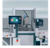
The intuitive layout is comprised of the control system, touch-screen monitor, scanner and the infeed and outfeed buffer conveyors. The operator can focus on the task without unnecessary distraction. For flexible production, all of our machines are individually adapted to customer requirements.
